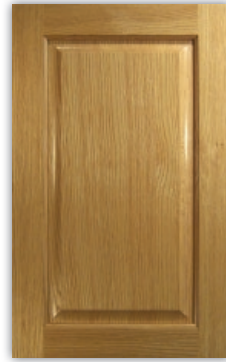
RED OAK RIFT CUT Cut at 30 to 60 degrees to the growth rings. Straighter grain than standard with wider more figured bands than 1/4 sawn.
